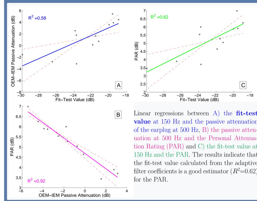
Linear regressions between A) the **fit-test value** at 150 Hz and the passive attenuation of the earplug at 500 Hz, B) the passive attenuation at 500 Hz and the Personal Attenuation Rating (PAR) and C) the fit-test value at 150 Hz and the PAR. The results indicate that the fit-test value calculated from the adaptive filter coefficients is a good estimator ( $R^2=0.62$ ) for the PAR.
