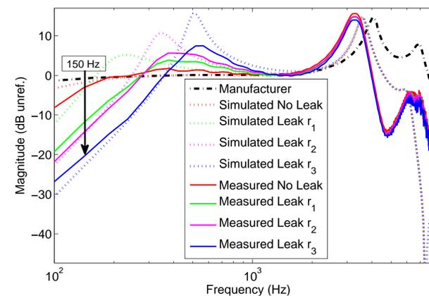
**Fig. 2:** Examples of different normalized miniature loudspeaker responses, with decreasing fit quality (acoustic leak equivalent diameter increasing from  $r_1$  to  $r_3$ ). The importance of the leak can be assessed by measuring the response magnitude around 150 Hz where the magnitudes differ the most between curves.
