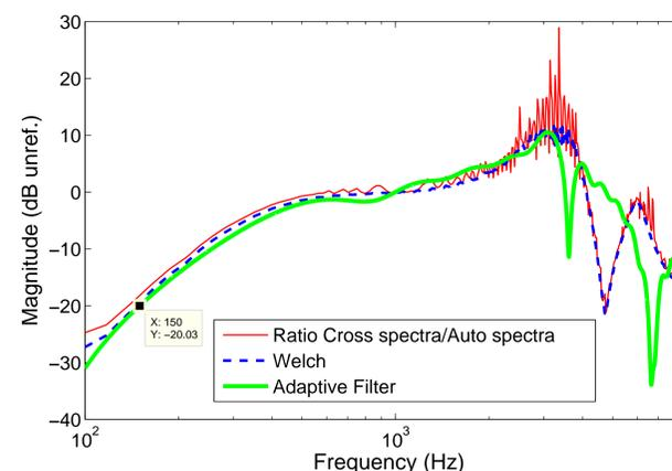
**Fig. 3:** Example of an estimate of the loudspeaker transfer function in low frequencies with the adaptive filter coefficients, similar to the transfer functions identified using the ratio of the cross spectra/auto spectra and the Welch estimator.
