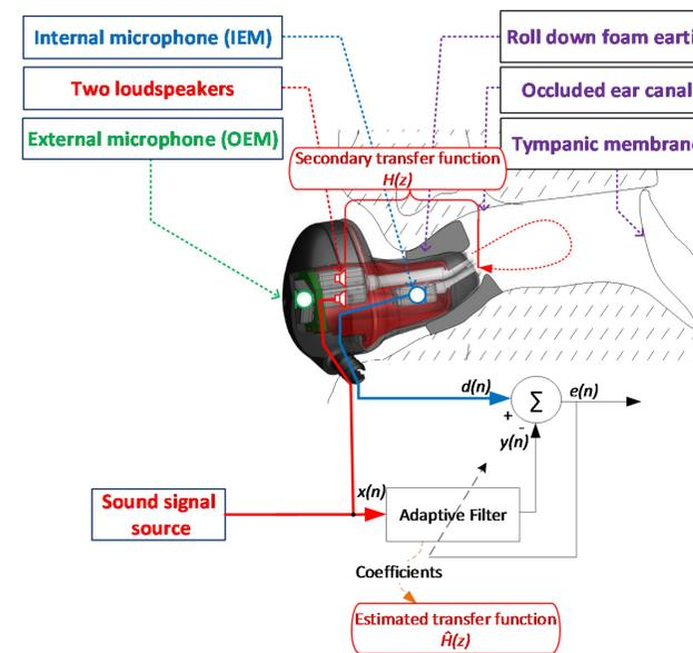
**Fig. 1:** Schematic of the procedure to identify the loudspeaker frequency response to evaluate the good fit of a hearing protector.
