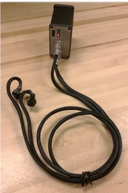
Fig. 1: The DPOAE measurement device designed in laboratory with its electronic hardware box and its two measurement probes featuring custom moulded ear-tips.
