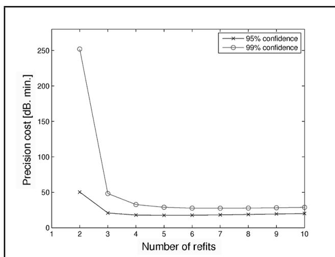
**Figure 5.** Precision cost according to the number of refits necessary for confidence intervals of 95% and 99%.
