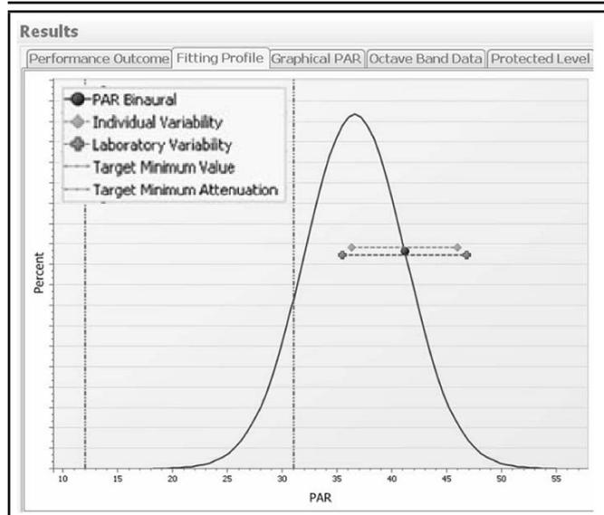
**Figure 6.** PAR value on the Results/Fitting Profile screen of SonoPass/EARfit software V3.2, clearly showing two error-bars accounting for both the F-MIRE measurement uncertainty and for the fit-variability: the fit-variability been assessed either on laboratory data (using the values presented in Fig. 5) or on individual data, if the subjects fits the earplug more than four times in a row.
