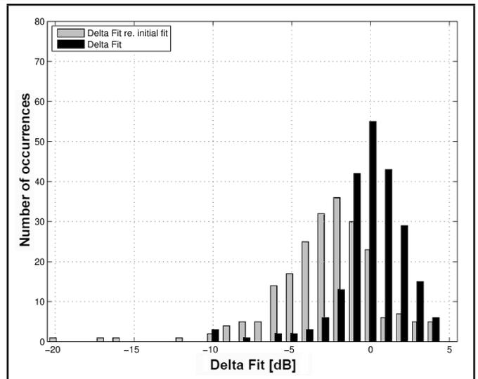
**Figure 3.** Histogram of the distance to ear mean attenuation  $\Delta FIT$  (in black) and of the distance to initial overall PAR attenuation  $\Delta FIT_{init}$  (in gray).
