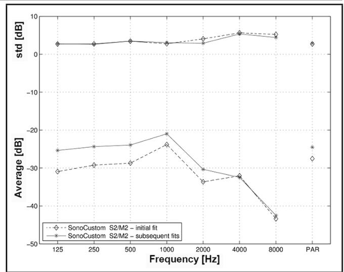
Figure 2. Average and standard deviation of the initial fit attenuation (in dotted line) and of the average of the 10 subsequent fits (in solid line).
