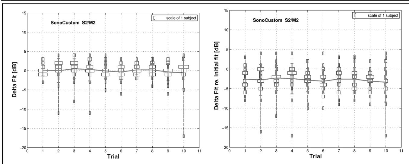
**Figure 4.** Average (solid gray line), standard deviation (gray vertical error bar) and histogram (gray bars) of the distance to overall ear mean attenuation for each of the ten trials (left chart) and of the distance to overall initial attenuation for the custom earplug (right chart).
