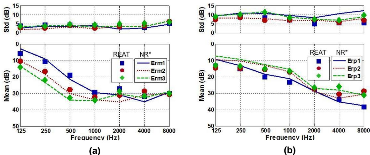
Figure 4: Comparisons of *REAT* (symbols) and *NR\** (lines) values for: a) the three earmuffs tested; b) the three earplugs tested. Mean and standard deviation values are shown (average over subjects)
