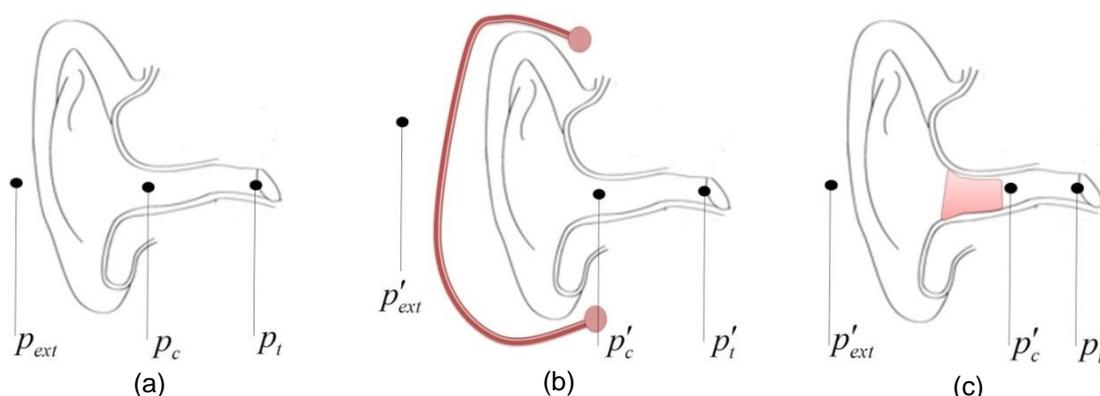
Figure 1: Illustration of the various microphone locations for the different ear conditions: a) open ear; b) occluded ear with an earmuff; c) occluded ear with an earplug
