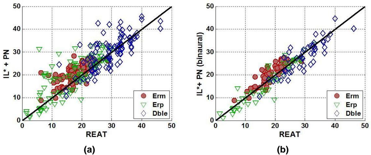
Figure 5: Comparisons of *PAR* values computed using  $AV=IL^*+PN$  and  $AV=REAT$  in equation (11): a) left and right ear results for  $IL^*$  results; b) left and right ear combined for  $IL^*$  results (binaural estimate). Results are presented in three groups: earmuffs (Erm), earplugs (Erp) and double protection (Dble).
