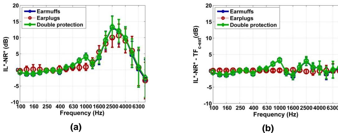
Figure 3: Differences between  $IL^* - NR^*$  for the three hearing protection condition tested: earmuffs (N=106), earplugs (N=106) and double protection (N=101)
