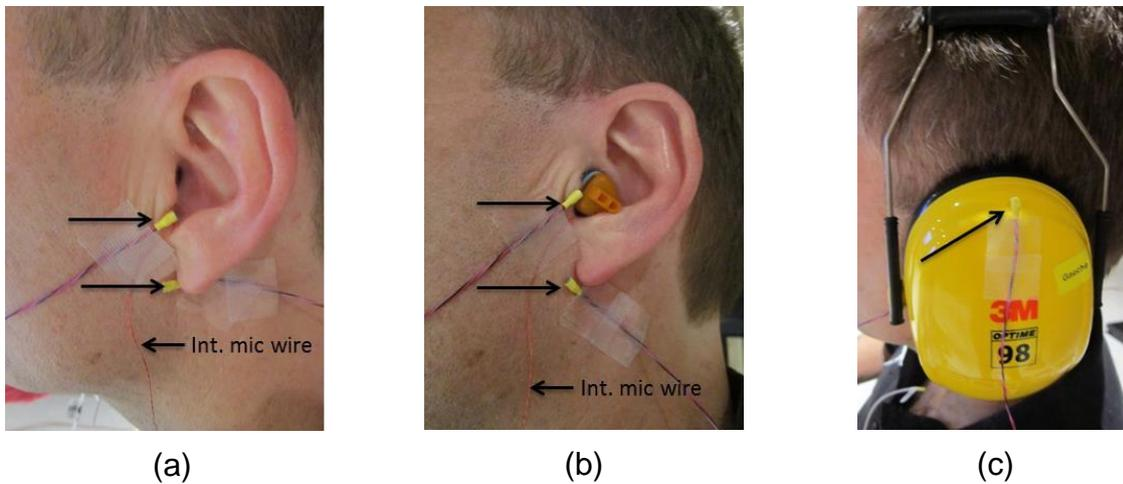
Figure 2: Locations of the microphones for the different conditions: a) unoccluded; b) earplugs; c) earmuffs. For the microphone located in the ear canal, only the connecting wire can be seen.
