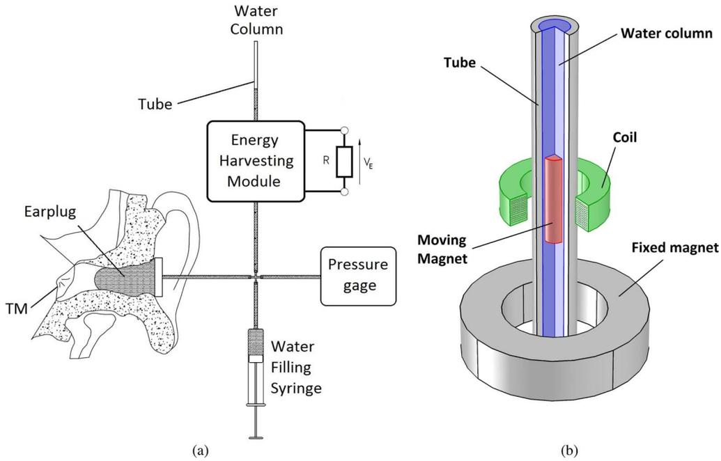
Fig. 3. Hydroelectromagnetic energy harvester. (a) Test setup. (b) Energy harvesting module.
