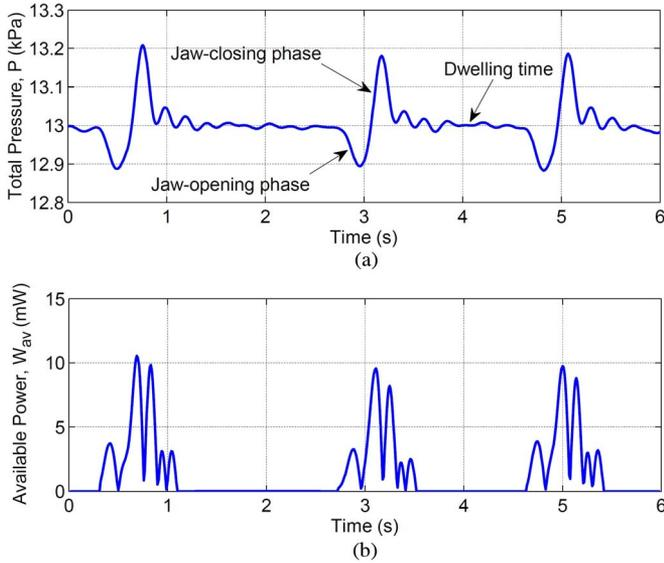
Fig. 4. Ear canal dynamic evaluation results. (a) Total pressure in the main column after applying a low-pass filter. (b) Available power during opening and closing of the mouth.
