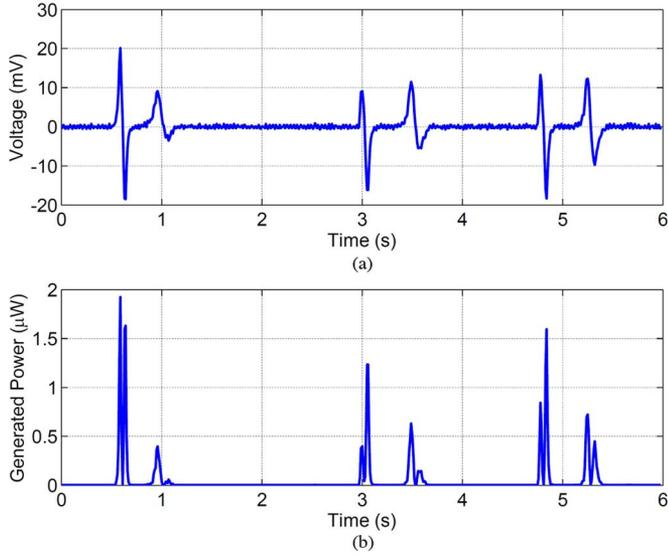
Fig. 6. Experimental results for the hydroelectromagnetic energy harvesting system. (a) Load voltage. (b) Generated power.
