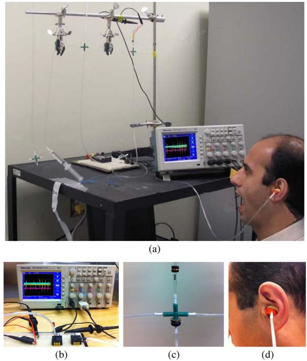
Fig. 5. Experimental setup for the hydroelectromagnetic energy harvesting system. (a) Overall view. (b) Pressure gauges and load resistance. (c) Energy harvesting module. (d) Expandable earplug in the ear canal.
