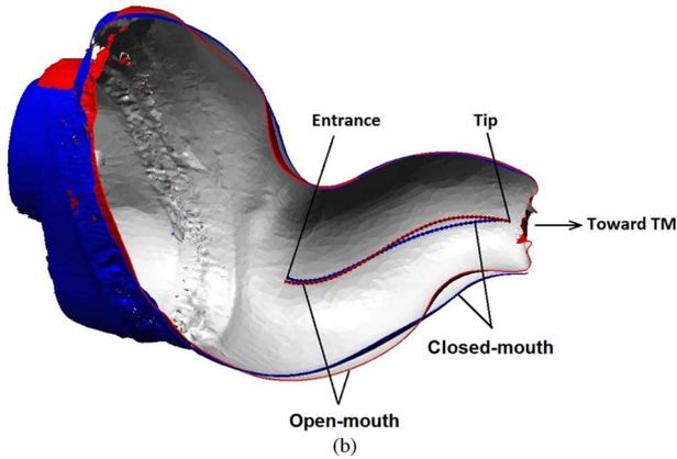
Fig. 2. Earplug geometries in *open-mouth* and *closed-mouth* positions. (a) Ear canal geometry. (b) Earplugs overlay.
