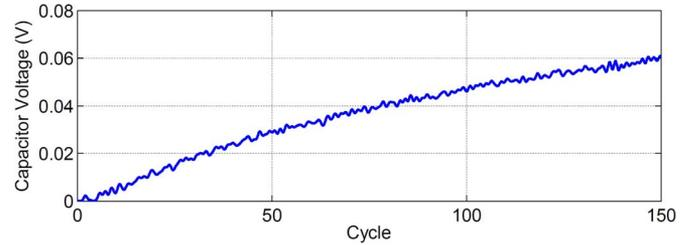
Fig. 8. Charging of a 24- $\mu\text{F}$  capacitor by the piezoelectric ring energy harvester during 150 cycles of opening and closing of the mouth.
