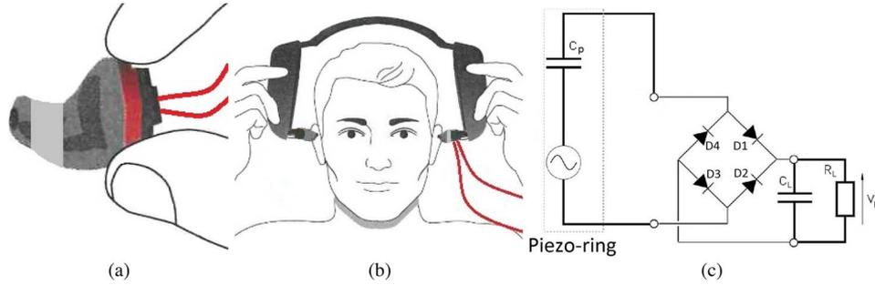
Fig. 7. Experimental setup for the piezoelectric energy harvesting system. (a) Earplug and piezoelectric ring. (b) Headset. (c) Capacitor charging circuit.
