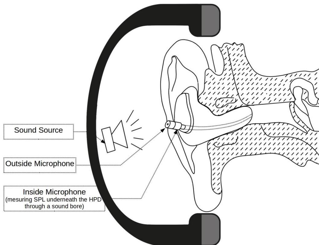
Figure 2: Illustration of an objective fit-test system using a microphone doublet under earphones to estimate the attenuation of a custom-molded earplug
