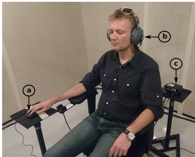
FIG. 1. (Color online) Subject wearing the HPs (b) and adjusting the mouse wheel (a) used for loudness equalization in the audiometric sound booth. The earpieces are fitted onto the subject's ears, under the HPs, and the microphones are connected to the battery-powered signal conditioning box (c) behind the subject.
