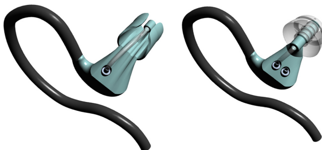
FIG. 3. (Color online) Three-dimensional models showing the OTE (left) and the CTE (right). In-ear measurements are performed via thin probe tubes connected to miniature electret microphones. An outer-ear microphone (OEM) on the CTE makes it possible to measure earplug attenuation.
