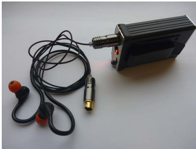
Fig. 8 The auditory research platform in which the VAD is implemented for real-time processing connected to two earpieces for audio signal acquisition and VAD's decision transmission.
