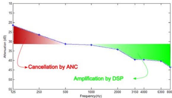
**FIGURE 8:** Example of achieving uniform attenuation: Since passive attenuation is usually the lowest in the low frequency region, using active noise control in that region will flatten the attenuation. A DSP could then be used to amplify high frequencies and achieve uniform attenuation in that region as well.
