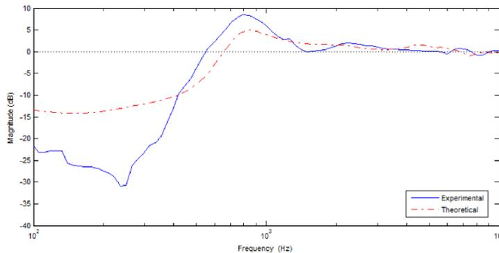
**FIGURE 11:** Active attenuation: the dashed line shows the expected active attenuation from theory and design. The solid line shows the measured active attenuation. Differences between the curves could be attributable to the variability of the acoustic seal which could in fact influence the *plant* response and therefore the performance of the system.
