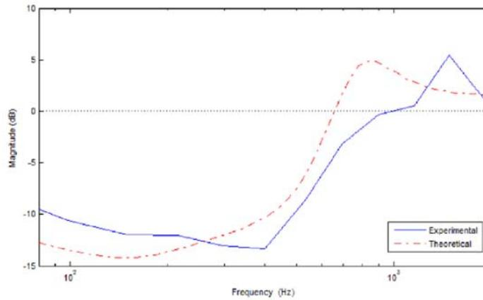
**FIGURE 10:** Occlusion effect cancellation: the dashed line shows the expected occlusion effect reduction from theory and design. The solid line shows the achieved occlusion effect cancellation for the first author.
