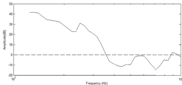
**FIGURE 2:** Occlusion effect: transfer function between an internal microphone, inside the occluded ear canal, and an external microphone, at the orifice of the ear canal, as the author is humming. The figure shows an estimation of the sound pressure increase caused by the occlusion effect. The sound pressure is seen to increase as high as 40 dB in the lower frequencies.
