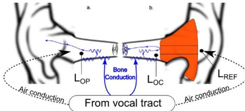
**FIGURE 1:** Occlusion effect: a) the sound wave induced by the vibration of the ear canal walls mostly escapes the ear canal and the sound wave travelling along the air conduction path is predominantly heard b) the trapped sound wave propagating from the bone conduction path will cause the eardrum to vibrate, while the air conduction path is blocked, causing an unnatural and augmented perception of one's own voice.
