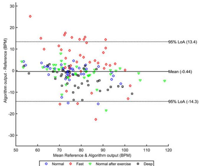
Fig. 8. Bland-Altman plot of heart rate extraction, showing good predictive capabilities of the algorithm on a wide range of BPM (mouth and nose breathing are both plotted but have the same symbol).
