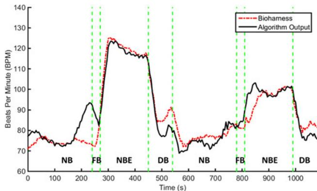
Fig. 7. Comparison between the reference heart rate and the output of the algorithm developed for 8 types of respiration over 18 minutes (in one ear), showing general good agreement between the two curves, with a mean absolute error of 4.0 BPM. Vertical lines indicate separations between the respiration types: four mouth breathing followed by four nose breathing.
