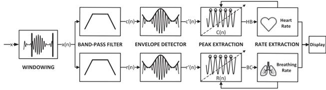
Fig. 5. Simplified block diagram of the heart and breathing rate extraction algorithms, showing the low complexity of the proposed algorithms.
