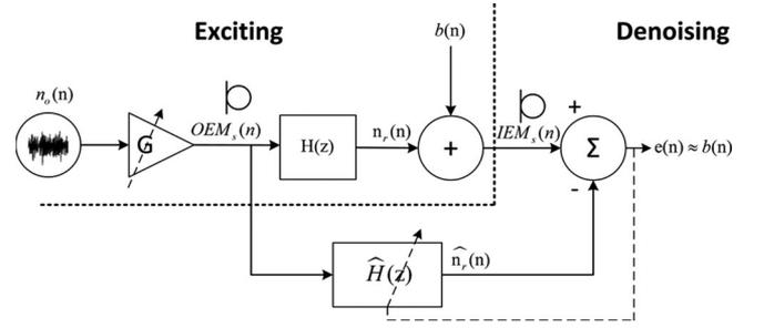
Fig. 6. Block diagram of adaptive filtering, showing the excitation portion, where industrial noise is added, and the denoising portion, where industrial noise is removed from the audio signal measured in the occluded earcanal.
