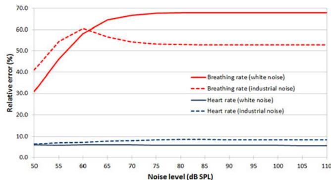
Fig. 11. Evolution of relative error averaged for 20 subjects as a function of noise level, showing good performance for heart rate extraction with white and industrial noise. The increase in the error is much greater for breathing rate extraction than for heart rate.
