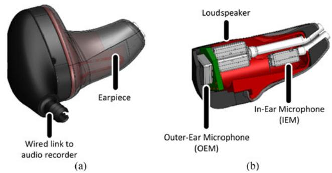
Fig. 1. Instrumented earpiece worn by each subject in each ear: (a) Intra-aural earpiece, (b) electroacoustic components.
