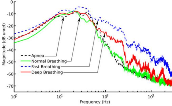
Fig. 4. Spectra of four types of nose respiration for one subject, showing different spectral characteristics to distinguish respiration types.
