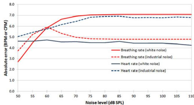
Fig. 10. Evolution of absolute error averaged for 20 subjects as a function of noise level, showing good performance for heart rate extraction with broadband white and industrial noise. The increase in the error is greater for breathing rate extraction with white and industrial noise.
