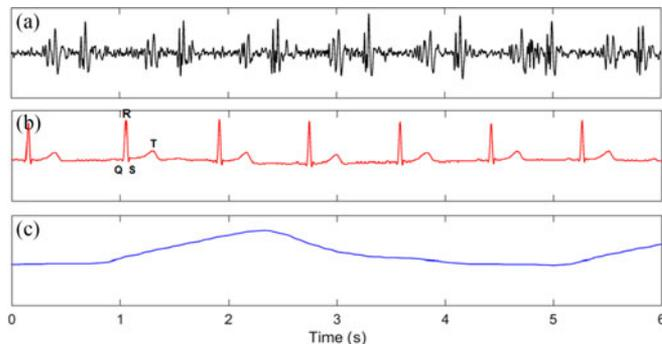
**Fig. 2.** (a) Time signal recorded by the IEM, showing events correlated to S1 and S2. Respiration is weak and almost non-measurable by the IEM. (b) Heartbeat reference recorded by the Bioharness, which is an electrocardiogram. A delay delay of less than 125 ms between audio data and Bioharness data may exist. (c) Respiration reference recorded by the Bioharness, which is a respiratory inductance plethysmography showing inspiration (ascending phase) and expiration (descending phase).
