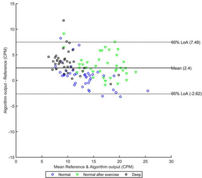
Fig. 9. Bland-Altman plot of the breathing rate extraction, showing good predictive capabilities of the algorithm on a breathing rate of fewer than 30 CPM (mouth and nose breathing are both plotted but are represented by the same symbol).
