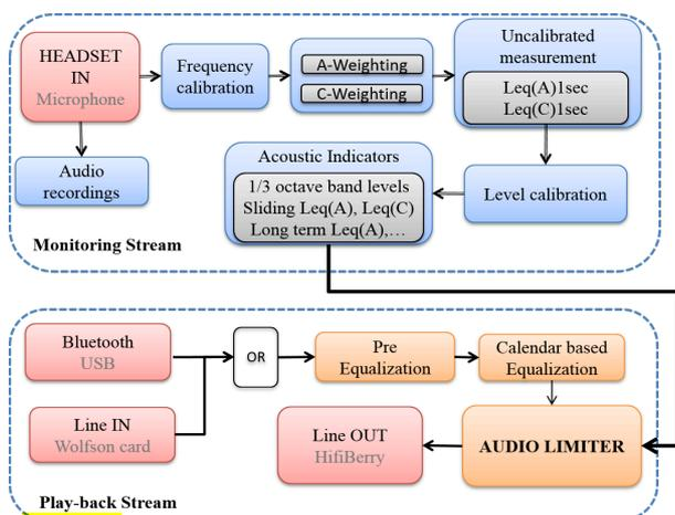
Figure 2: Audio processing components of monitoring and playback streams
