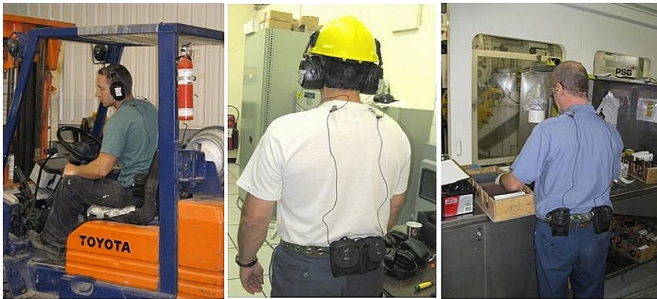
Fig. 2. Examples of workers equipped with two sets (one per ear) of measurement systems. This figure appears in color online.
